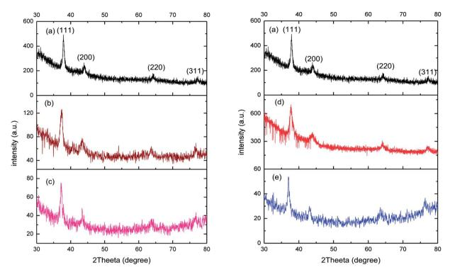
Fig. 7 XRD pattern for (a) bare PVP-AgNPs, (b) 0.05 mM Amk@PVP-AgNPs, (c) 0.3 mM Amk@PVP-AgNPs, (d) 0.05 mM Van@PVP-AgNPs and (e) 0.3 mM Van@PVP-AgNPs
