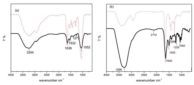
Fig. 4 FTIR spectra of (a) Amk@PVP-AgNPs (dotted line) and amikacin (solid line) and (b) Van@PVP-AgNPs (dotted line) and vancomycin (solid line).
