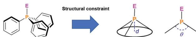
Fig. 36 Schematic representation of triphenylphosphine and its axially occupied derivatives. The bowl depth ( d ) and the cone angle ( \theta ) represent the key parameters when structural constraining the parent structure. 27 Figure reproduced with kind permission; © 2019 American Chemical Society.
