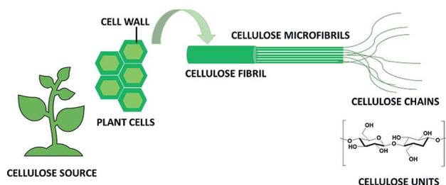
Fig. 1 Schematic representation of cellulose fibrils and microfibrils.
