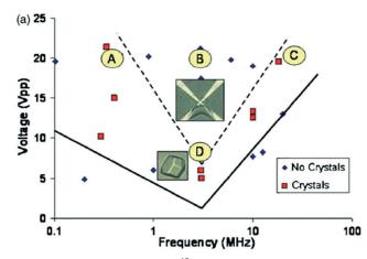
**Fig. 3** Results of Hou and Chang<sup>15</sup> of HEWL solutions in the presence of different internal AC fields, having been observed for 24 hours for signs of nucleation. A and C are within the crystallization window during this time, while gelation takes place for B. The point D indicates the frequency, where the lowest voltage is required for crystallization. Reprinted from ref. 15 with the permission of AIP Publishing.
