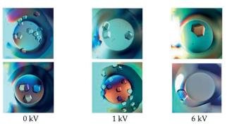
Fig. 2 Glucose isomerase crystals grown under the application of a DC electric field of varying intensities. Each row corresponds to experimental results obtained on different dates.<sup>17</sup> Reprinted with permission from ref. 17 Copyright (2017) American Chemical Society.
