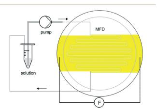
Fig. 6 Continuous flow electric-field assisted crystallization process flow diagrammatic setup of Li and Lakerveld. 54 Reprinted with permission from ref. 54 Copyright (2018) American Chemical Society.
