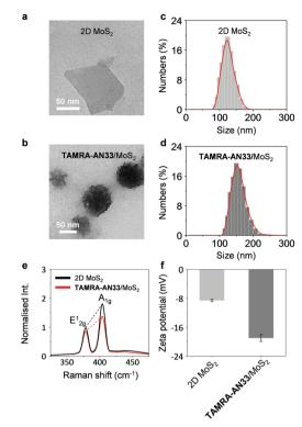
Fig. 2 HRTEM images of (a) 2D MoS<sub>2</sub> (30 μg mL $^{-1}$ ) and (b) **TAMRA-AN33**/MoS<sub>2</sub> (5 μM/30 μg mL $^{-1}$ ). DLS of (c) 2D MoS<sub>2</sub> (30 μg mL $^{-1}$ ) and (d) **TAMRA-AN33**/MoS<sub>2</sub> (5 μM/30 μg mL $^{-1}$ ). (e) Raman spectra of 2D MoS<sub>2</sub> (30 μg mL $^{-1}$ ) and **TAMRA-AN33**/MoS<sub>2</sub> (5 μM/30 μg mL $^{-1}$ ). (f) Zeta potential of 2D MoS<sub>2</sub> (30 μg mL $^{-1}$ ) and **TAMRA-AN33**/MoS<sub>2</sub> (5 μM/30 μg mL $^{-1}$ ).
