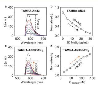
Fig. 3 (a) Fluorescence spectra and (b) titration of **TAMRA-AN33** (0.25  $\mu$ M) with increasing 2D MoS<sub>2</sub> (0–30  $\mu$ g mL<sup>-1</sup>); (c) fluorescent spectra and (d) titration of **TAMRA-AN33** (0.25  $\mu$ M) complexed with 2D MoS<sub>2</sub> (30  $\mu$ g mL<sup>-1</sup>) with increasing PROCR protein (0–110 nM); the solvent used is PBS (0.01 M, pH 7.40). Excitation wavelength = 530 nm.
