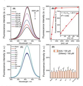
Fig. 2 The analytical performance and selectivity of this sensor for AA detection. (A) and (B) Fluorescence spectra and calibration curve for AA detection. Inset: A linear relationship of the fluorescence signal versus the concentration of AA ranging from 0 to 800  $\mu M$ . (C) and (D) Fluorescence spectra and fluorescence signal of different interferents. All concentrations were 100  $\mu M$ . Error bars were estimated from at least three replicate measurements.
