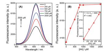
Fig. 3 The analytical performance of this ascorbic acid sensor in 1% fruit juice solution. (A) Fluorescence emission spectra of the biosensor upon the addition of different concentrations of AA. (B) Calibration curve with the inset showing the linear relationship of the fluorescence signal versus the concentration of AA ranging from 0.5 to 800  $\mu\text{M}$ . Error bars were estimated from three replicate measurements.
