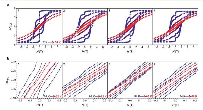
Fig. 5 (a) Magnetic hysteresis data for 1-4 collected at 2, 10, 20 and 30 K with a sweep rate of 3.1(4) mT s<sup>-1</sup> for H < 2 T and 13.2(2) mT s<sup>-1</sup> for H > 2T. (b) Expanded view of the region near zero field at high-temperatures.
