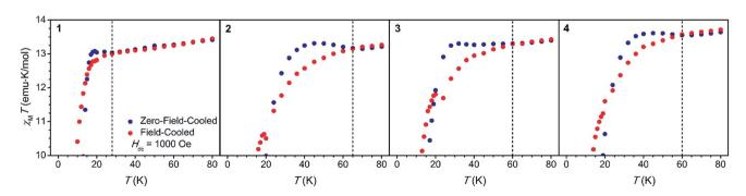
Fig. 2 Field-cooled (red) and zero-field cooled (blue) magnetic susceptibility measurements collected at  $H_{dc} = 1000$  Oe for 1–4 (left to right). Dashed lines mark  $T_{irrev}$ , the temperature at which the two plots diverge.
