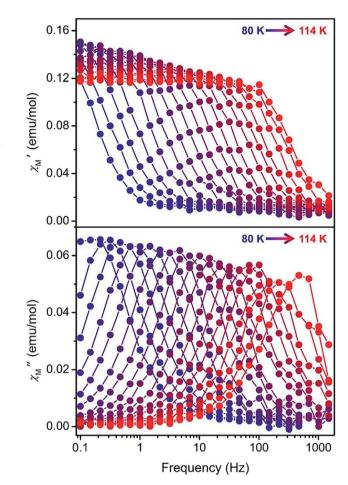
Fig. 3 In-phase ( $\chi'_{M}$ , top) and out-of-phase ( $\chi''_{M}$ , bottom) components of the ac magnetic susceptibility for 2 under zero applied dc field at frequencies ranging from 0.1–1500 Hz and temperatures from 80–114 K (2 K steps). The colored lines are guides for the eye.
