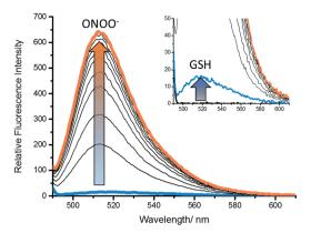
Fig. 2 Fluorescence spectra of GSH-PF3 (0.5 μM) with addition of GSH (200  $\mu$ M), 10 min wait (inset), then addition of ONOO<sup>-</sup> (0–10  $\mu$ M) in buffer solution [52 wt% methanol] (pH = 8.21 at 25  $^{\circ}$ C). Fluorescence intensities were measured with  $\lambda_{ex} = 488$  nm with slit widths ex slit: 5 nm and em slit: 2.5 nm.
