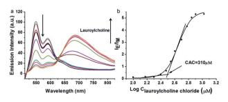
Fig. 1 (a) Changes in emission spectra of PDI-DHA (10  $\mu$ M) in the presence of different concentrations  $(0-800 \mu M)$  of lauroylcholine. (b) Corresponding  $I_{\text{E}}/I_{\text{M}}$  value changes of PDI-DHA (10  $\mu\text{M}$ ) as a function of lauroylcholine concentration.
