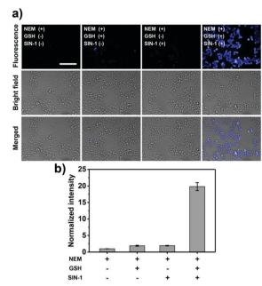
Fig. 4 Fluorescence imaging (a) and quantification (b) of RAW264.7 cells with **GSH-ABAH** (20  $\mu$ M) in the presence of exogenously added GSH (300  $\mu$ M) and/or SIN-1 (500  $\mu$ M) with 1% DMSO. Excitation channel 360–400 nm, emission channel filtered = 410–480 nm. Scale bar = 100  $\mu$ m. Error bars represent SD. Note: the cells were pre-incubated with *N*-ethylmaleimide (NEM, GSH scavenger).
