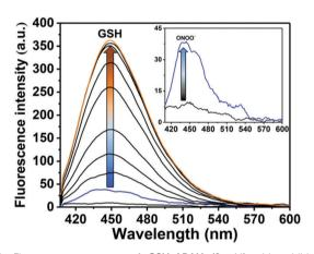
Fig. 2 Fluorescence spectra of GSH-ABAH (2 μM) with addition of ONOO<sup>-</sup> (4  $\mu$ M) (inset) followed by the addition of GSH (0-2  $\mu$ M), and 1 min wait in buffer solution [8% DMSO, 1 mM CTAB] (pH = 8.20 at 25 °C) fluorescence intensities were measured with  $\lambda_{ex}$  = 390 nm/ $\lambda_{em}$  = 451 nm with slit widths ex slit: 4 nm and em slit: 4 nm.
