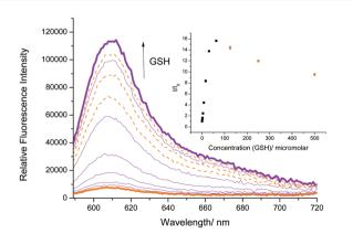
Fig. 2 Fluorescence spectra of TCF-GSH (5  $\mu$ M) with addition of GSH  $(0-500 \mu M)$  and 15 min wait between additions in PBS buffer solution, 20% v/v DMSO, pH 8.00 at 25 °C.  $\lambda_{ex}$  = 560  $\pm$  15 nm. Orange dashed lines indicate fluorescence decrease at high GSH concentrations.
