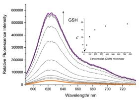
Fig. 3 Fluorescence spectra of TCFCl-GSH (5  $\mu$ M) with addition of GSH (0-750 μM) and 15 min wait between additions in PBS buffer solution, 20% v/v DMSO, pH 8.00 at 25 °C.  $\lambda_{\rm ex}$  = 560  $\pm$  15 nm.
