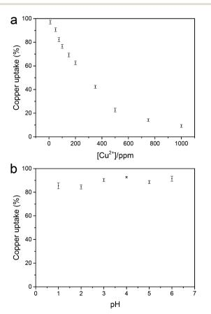
Fig. 3 (a) Metal uptake as a function of Cu(II) ion concentration and (b) metal uptake of the NGC membrane as a function of pH ( $[Cu^{2+}] = 50 \text{ mg L}^{-1}$ ).
