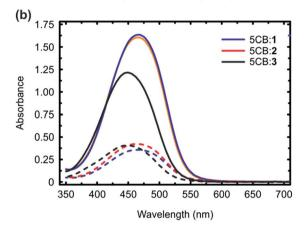
Fig. 2 (a) Isotropic-to-nematic phase transition temperatures as a function of dye doping for the 5CB:x systems, as determined by DSC. (b) Polarized absorption spectra of the 5CB:x systems with 1 mol% dye concentration in planar LC cells with 10  $\mu$ m thickness, illustrating that the order parameter of the dyes in 5CB develops in the order 1 > 2 > 3. The solid and dashed lines correspond to spectra measured along and perpendicular to the LC director, respectively.
