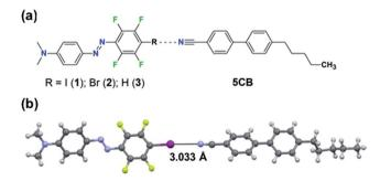
Fig. 1 (a) Chemical structures of the studied systems. (b) Crystal structure of the halogen-bonded complex between 1 and 5CB. For clarity, only the most populated conformer of each molecule is shown.
