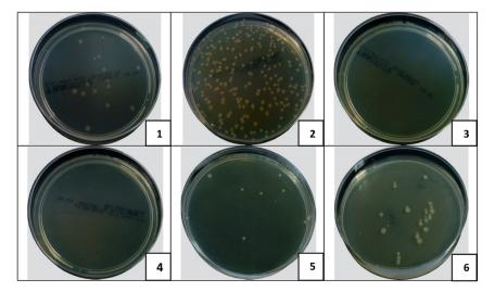
Fig. 9 Images of agars after the testing of bacterial filtration efficiency and after the "smear-test" for pristine PU fibers and for composite fibers: (1) PU filtration; (2) PU smear test; (3) 9.5% of micro CuO, filtration; (4) 9.5% of micro CuO, smear test; (5) 9.5% of nano CuO, filtration; (6) 9.5% of nano CuO, smear test.
