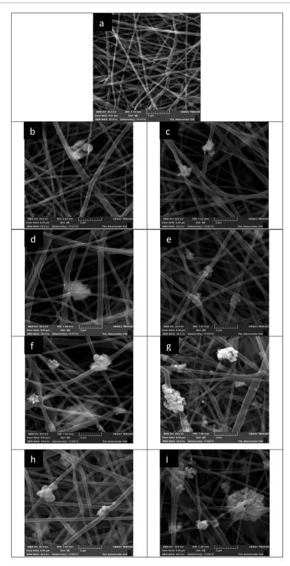
Fig. 4 SEM images (magnification 20 000) of nanofibers with different concentrations of micro- or nanoparticles of CuO: (a) 0%; (b) 5%  $\mu$ m; (c) 5% nm; (d) 7%  $\mu$ m; (e) 7% nm; (f) 9.5%  $\mu$ m; (g) 9.5% nm; (h) 12%  $\mu$ m; (i) 12% nm.
