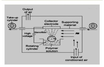
Fig. 1 Schematic diagram of the Nanospider method.
