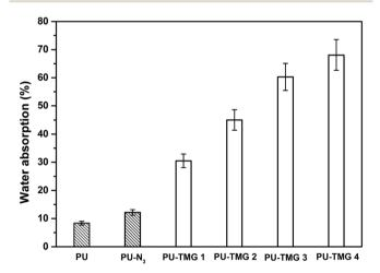
Fig. 8 Water absorption properties of PU, PU-N<sub>3</sub>, PU-TMG 1 (wt% = 0.6%), PU-TMG 2 (wt% = 1.0%), PU-TMG 3 (wt% = 2.1%), and PU-TMG 4 (wt% = 5.5%) at room temperature for 72 hours.
