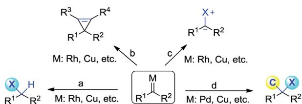
Scheme 1 Representative reaction modes of a transition-metal carbenoid.
