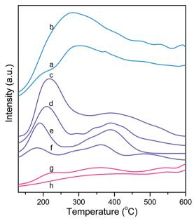
Fig. 4 NH<sub>3</sub>-TPD curves of the fresh aluminosilicate catalysts: (a) SA@0.03, (b) SA@1.79, (c) ZSM-5@30, (d) ZSM-5@64, (e) ZSM-5@106, (f) ZSM-5@260, (g) Al-SBA-15@102 and (h) Al-SBA-15@190
