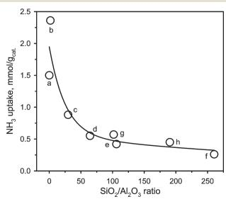
Fig. 5 Evolution of the total acidity on the fresh aluminosilicate catalysts measured by NH<sub>3</sub>-TPD as a function of the SiO<sub>2</sub>/Al<sub>2</sub>O<sub>3</sub> ratio: (a) SA@0.03, (b) SA@1.79, (c) ZSM-5@30, (d) ZSM-5@64, (e) ZSM-5@106, (f) ZSM-5@260, (g) Al-SBA-15@102 and (h) Al-SBA-15@190.
