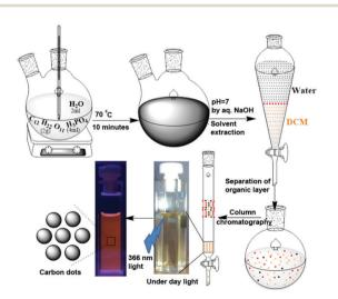
Scheme 1 Preparation and purification of orange-red emitting carbon dots using sucrose and H<sub>3</sub>PO<sub>4</sub>.
