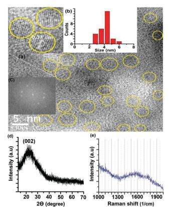
Fig. 2 (a) TEM image (HRTEM image in inset), (b) size distribution histogram, (c) fast Fourier transform pattern of the HRTEM image, (d) XRD pattern and (e) Raman spectrum of the S-CDs.
