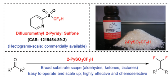
Fig. 1 Difluoromethyl 2-pyridyl sulfone and its carbonyl gem -difluoroolefination reaction.
