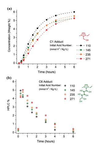
Fig. 11 Comparison of adduct formation for  $[C_2C_1\text{im}][OAc]$ , 1a + 10 wt% D-(+)-glucose, 12, with differing initial acid numbers (110-271 mmol H<sup>+</sup> kg<sup>-1</sup> IL), heated at 120 °C for 24 hours: (a) wt% of the C1 adduct,  $[C_2C_1(HO)C_1^2\text{im}]^+$ ; (b) HPLC% of the intermediate C6 adduct. Graphs are shown in the range  $t_0-t_6$ , for clarity.
