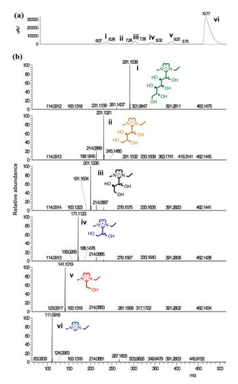
Fig. 4 LCMS investigation of adduct species formed from [C2C1im]-[OAc], 1a + 10 wt% D-(+)-glucose, 12, heated to 120 °C for one hour ( $t_1$ ): (a) survey of peaks i-vi; (b) ESI mass spectra of peaks i-vi.
