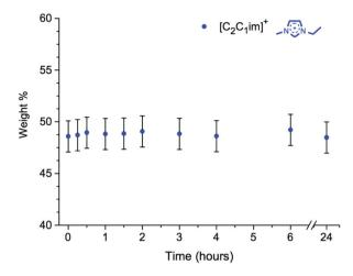
Fig. 12 Wt% concentration of  $[C_2C_1\text{im}]^+$  during the heating of  $[C_2C_1\text{im}][CH_3SO_3]$ , 3 + 10 wt% D-(+)-glucose, 12, at 120 °C for 24 hours. Error values are approximate, based upon the largest errors for triplicate experiments of  $[C_2C_1\text{im}][OAc]$ , 1a + 10 wt% 12.
