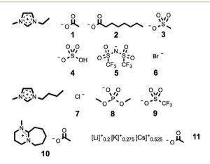
Fig. 1 lonic liquids used in this study, incorporating the  $[C_2C_1im]^+$  (1–6),  $[C_4C_1im]^+$  (7–9), and  $[Me-DBU]^+$  (10) cations. Compound 11 is a low-melting mixed inorganic eutectic salt.
