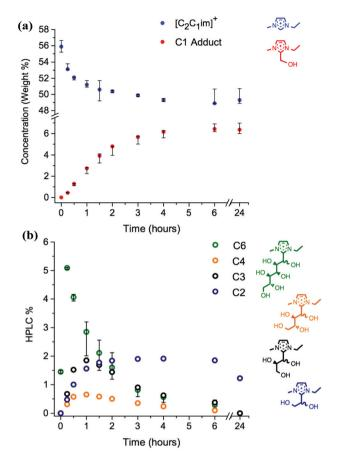
Fig. 3 1-Ethyl-3-methylimidazolium acetate,  $[C_2C_1\mathrm{im}][OAc]$ , 1a+10 wt% D-(+)-glucose, 12, heated to 120 °C for 24 hours: (a) wt% of the  $[C_2C_1\mathrm{im}]^+$  cation and the 'C1' adduct cation,  $[C_2C_1(HO)C_1^{-2}\mathrm{im}]^+$ . (b) HPLC% concentrations of the 'intermediate' C6–C2 adducts. Error bars for C4–C2 adducts are omitted for clarity, but are typically < $\pm$ 0.2 HPLC%.
