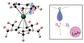
Fig. 8 Molecular structure of [Er(Cp\*)(COT)] (left) and a schematic depiction of the physical meaning of the radial  $(D_r)$  and vertical  $(D_v)$  displacement parameters (right). Reprinted with permission from ref. 25. Copyright 2014 American Chemical Society.
