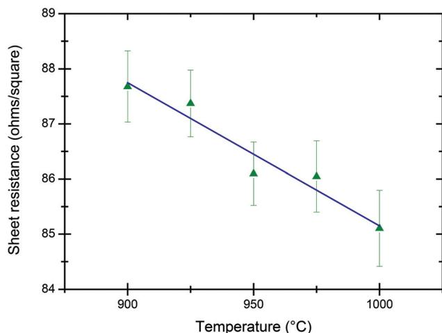
**Fig. 5** Sensitivity of sheet resistance to anneal temperature. 3 minutes RTA at various temperatures. The same indicated implanted fluence of  $10^{15} \text{ As cm}^{-2}$  is used here with all the 5 implants done at the same time. The vertical error bars are given as the standard deviation of 197 measurements performed on each wafer. Linear regression is also shown on the figure (blue line).
