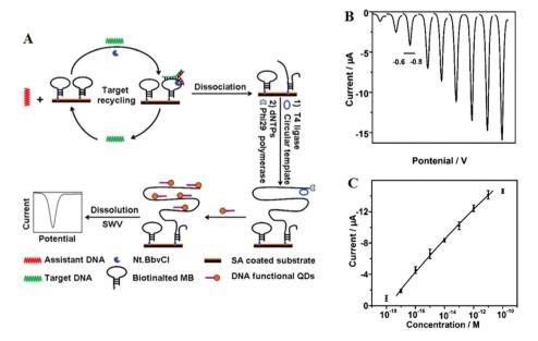
Fig. 6 (A) Schematic illustration of the TEHP amplification strategy for DNA detection, (B) stripping voltammetric curves of cadmium ions corresponding to (left to right)  $10^{-18}$ ,  $10^{-16}$ ,  $10^{-15}$ ,  $10^{-14}$ ,  $10^{-13}$ ,  $10^{-12}$ ,  $10^{-11}$ , and  $10^{-10}$  M of target DNA. (C) The corresponding analytical quantitative dynamic range. Reprinted permission from ref. 46, copyright@2012, American Chemical Society.
