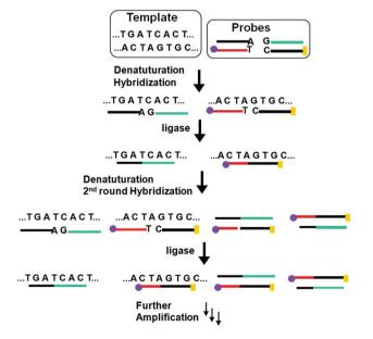
Fig. 3 Schematic principle of the ligase chain reaction (LCR) based DNA amplification strategy. Each of the two DNA strands in the duplex target serves as a template to ligate its respective two short DNA strands, leading to doubling of the ligated product in each cycle and hence an exponential amplification of the target DNA. The amplified target sequences can then be detected by using their specific • and • tags.
