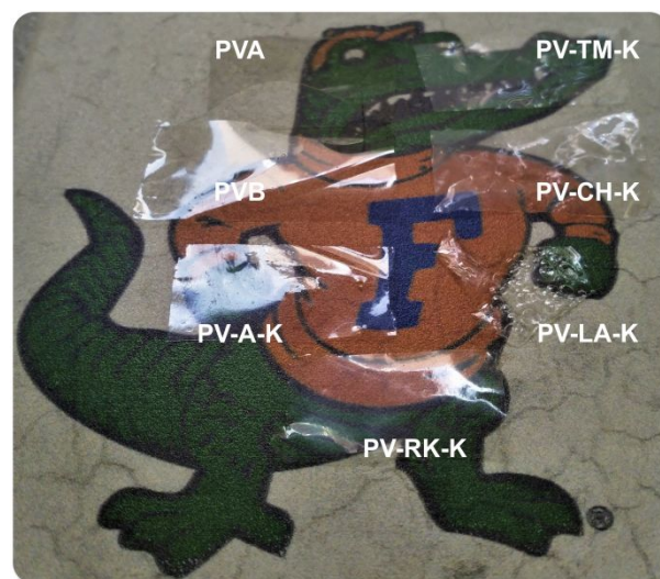
Fig. 8. Films from PV-A-K , PV-RK-K , PV-TM-K , PV-CH-K , and PV-LA-K exhibit optical transparency comparable to that of films from commercial polyvinyl alcohol (PVA) and polyvinyl butyral (PVB).
