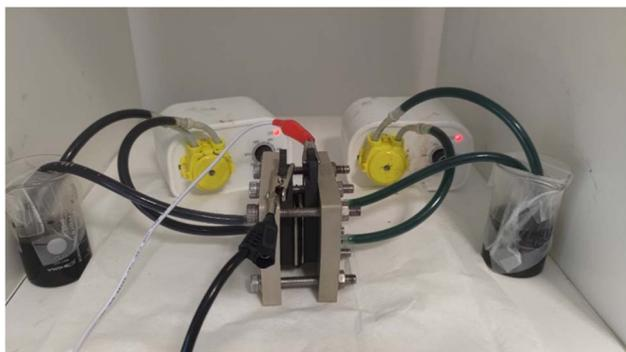
**Fig. 1** The general assembly of a redox flow battery comprising of two pumps, two beakers consisting of catholyte and anolyte (indicated by dark brown (+5), and green (+2) respectively), and a cell stack consisting of porous electrodes, membrane, and current collector plates.
