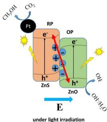
Fig. 11 Diagrammatic representation of the S-scheme mechanism of the photogenerated charge carrier transfer process, where  $\vec{E}$  denotes the electric field's direction. Drawn from scholarly sources (Mohamed *et al.*, 2021).
