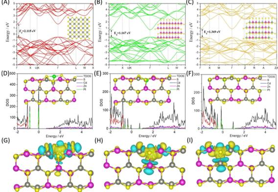
Fig. 12 The electronic structures of (A) ZnS, (B) CdS, and (C) ZnxCd1-xS are shown (the gray, pink, and yellow spheres represent Zn, Cd, and S atoms, respectively). The work functions of (D) ZnxCd1@xS-Pt1, (E) ZnxCd1@xS-Pt1 (Zn), (F) ZnxCd1@xS-Pt1 (Cd). (G), (H), and (I) indicate the DOSs and charge density differences. 139
