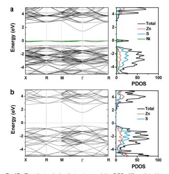
Fig. 13 The electronic band structure and the DOS; differentiated into total and partial. (a) ZnS that is 2.7% doped with Ni and (b) undoped ZnS.<sup>52</sup>
