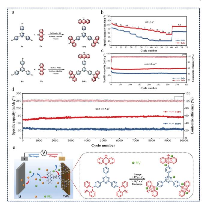
Fig. 16 (a) The synthetic reaction route of TzPz and BzPz. (b) The rate performance at current densities from 0.2 to 30 A  $g^{-1}$ . (c) Cycling performance at current densities of 0.2 A g<sup>-1</sup> and (d) 5 A g<sup>-1</sup>. (e) Schematic diagram of the electrochemical reaction mechanism of the TzPzbased cathode. 112 Copyright 2021, Wiley.
