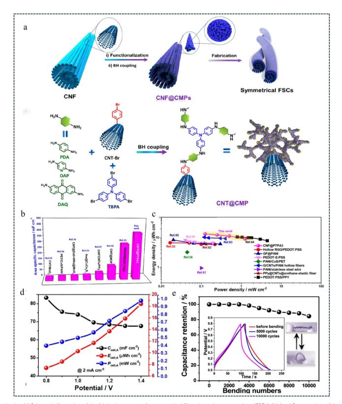
Fig. 21 (a) Schematic illustration of the fabrication process for symmetrical fiber-shaped supercapacitors (FSCs). (b) Areal Ragone plots of the CNF@PTPA-based FSCs. (c) Comparison of electrochemical performance of CNF@PTPA FSCs with other FSCs in terms of specific capacitance. (d) GCD curves of CNF@CMP fibers. (e) Relationship between capacitance retention and bending times. 131 Copyright 2020, American Chemical Society.
