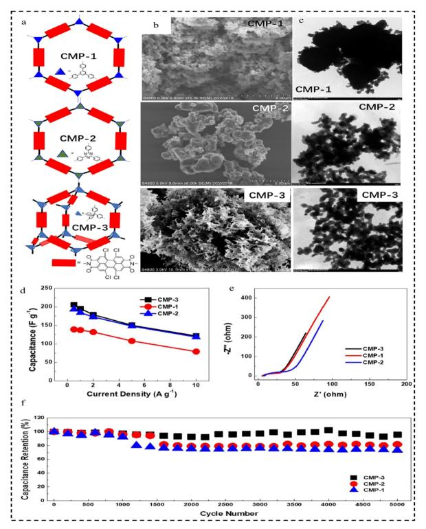
Fig. 19 (a) Graphic representation of CMP-1, CMP-2 and CMP-3. (b) SEM images of CMP-1, CMP-2 and CMP-3. (c) TEM images of CMP-1, CMP-2 and CMP-3. (d) Specific capacitance versus current density curve of CMP-1, CMP-2 and CMP-3. (e) Nyquist plot of CMP-1, CMP-2 and CMP-3. (f) Cycling stability of CMP-1, CMP-2 and CMP-3 at a current density of 10 A g<sup>-1</sup> <sup>125</sup> Copyright 2022, Springer.
