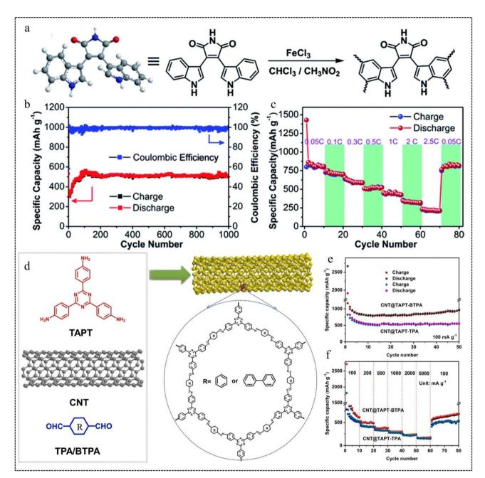
Fig. 6 Oxidative coupling polymerization routes. (a) Synthesis of PBIM. (b) Cycle performance of CMP-PBIM. (c) The rate performance at different current densities from 0.05C to 2.5C.<sup>67</sup> Copyright 2018, Royal Society of Chemistry. Schiff-base reaction routes. (d) Synthetic route of CNT@TAPT-TPA/BTPA. (e) Cycling performance of CNT@TAPT-TPA and CNT@TAPT-BTPA. (f) Rate performance of CNT@TAPT-TPA and CNT@TAPT-BTPA. (e) Copyright 2023, Elsevier.
