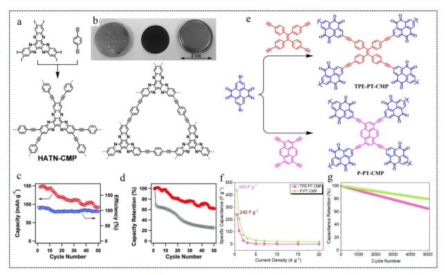
Fig. 2 (a) Synthesis of HATN-CMP networks. (b) The photos of HATN-CMP electrodes. (c) Cycle stability and (d) capacity retention ratio of HATN-CMP.<sup>44</sup> Copyright 2014, Royal Society of Chemistry. (e) Synthetic pathway of TPE-PT-CMP and P-PT-CMP. (f) Capacitance retention and (g) Ragone curve. 45 Copyright 2022, American Chemical Society.
