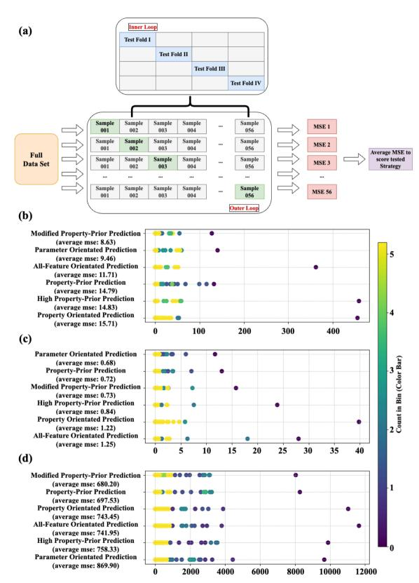
Fig. 8 (a) Evaluation of the ML strategy based on LOOCV and NCV, and visualized performance of Mean Squared Error (MSE) in predicting (b) photocatalytic NO conversion, (c) photocatalytic  $NO_x$  conversion and (d) photocatalytic  $NO_2$  selectivity in 56 NCV cycles for each ML strategy, where colours represent the number of times the MSE falls within this range.
