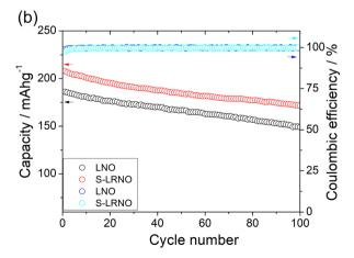
Fig. 7 (a) Initial charge-discharge curves LNO and S-LRNO synthesised by the co-precipitation route between 2 and 4.3 V at 25 mA  $\mbox{g}^{-1}$  (after the formation cycle). (b) The cycling performance of LNO and S-LRNO at 100 mA g<sup>-1</sup>
