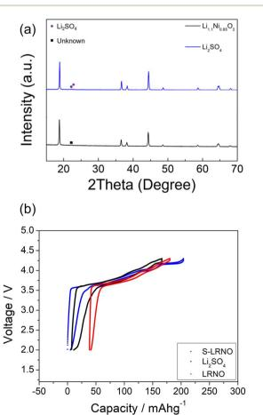
Fig. 6 (a) XRD patterns of  $Li_{1.1}Ni_{0.85}O_{2-x}$ , and  $Li_2SO_4$  ball milled  $Li_{1.1}$ - $Ni_{0.85}O_{2-x}$ . (b) Charge-discharge curves of solid state route synthesised LRNO, S-LRNO and LRNO with 5%Li<sub>2</sub>SO<sub>4</sub> between 2 and 4.3 V at 25 mA  $g^{-1}$  (after the formation cycle).
