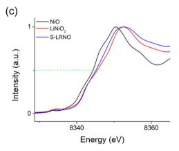
Fig. 2 (a) XRD patterns of Li $_{1.1}$ Ni $_{0.85}$ O $_2$ , Li $_{1.1}$ Ni $_{0.875}$ So $_{0.025}$ O $_{2-x}$  and Li $_{1.1}$ Ni $_{0.85}$ So $_{0.05}$ O $_{2-x}$  (solid state synthesis route). (b) Observed, calculated and difference profiles from structural refinement of Li $_{1.1}$ Ni $_{0.85}$ So $_{0.05}$ O $_{2-\delta}$  using neutron diffraction data (c) XAS data of Li $_{1.1}$ Ni $_{0.85}$ So $_{0.05}$ O $_{2-x}$ .
