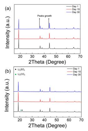
Fig. 4 XRD patterns of (a) LiNiO<sub>2</sub> and (b) Li<sub>1.1</sub>Ni<sub>0.85</sub>S<sub>0.05</sub>O<sub>2- $\delta$ </sub> (solid state route) after the exposure in air after 1, 15 and 30 days.
