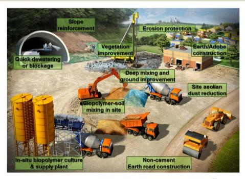
Fig. 10 Schematic representation of applications of biopolymers in the field of geotechnical engineering.<sup>136</sup> Reprinted with permission from Sustainability (2016).
