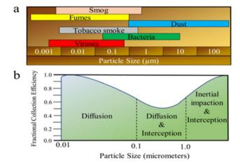
Fig. 15 (a) Size proportions of common air pollutants and (b) fractional collection effectiveness for various mechanical filters in relation to the contaminant diameter.<sup>150</sup> Reprinted with permission from ACS Publication (2021).
