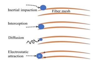
Fig. 14 Impaction, diffusion, interception, and electrostatic interaction are frequently used filtration mechanisms for biopolymers (orange lines). The pollutant, represented as a blue sphere, moves along a black path, and interactions between the pollutant and the biopolymer are shown as red dotted lines.<sup>150</sup>
