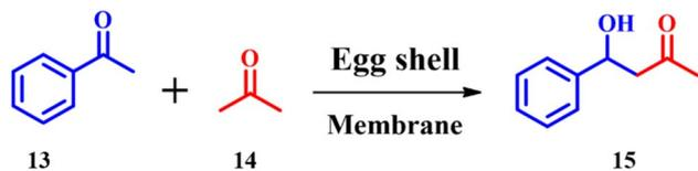
Scheme 6 Synthesis of 4-hydroxy-4-phenylbutan-2-one (adapted from ref. 38).
