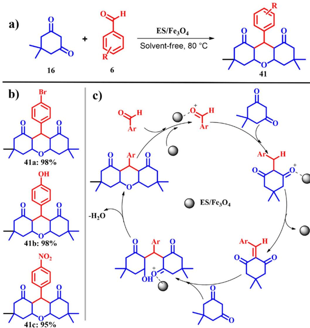
**Scheme 16** (a) and (b) Nano-ES/Fe<sub>3</sub>O<sub>4</sub>-catalyzed synthesis of 3,3,6,6-tetramethyl-9-phenyl-1,8-dioxo-1,2,3,4,5,6,7,8-octahydroxanthene and (c) proposed mechanism (adapted from ref. 54).
