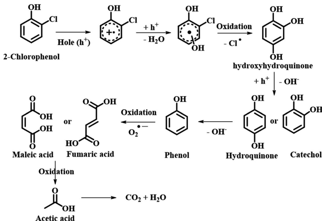
Scheme 23 Photocatalytic degradation pathway of 2-CP over 30Fe/QES (adapted from ref. 84).
