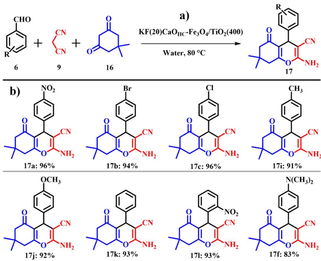
Scheme 8 (a) KF(20)CaO<sub>HFC</sub>-Fe<sub>3</sub>O<sub>4</sub>/TiO<sub>2</sub>(400) catalyzed one-pot synthesis of tetrahydro-4*H*-chromenes and (b) tetrahydro-4*H*-chromene derivatives (adapted from ref. 42).
