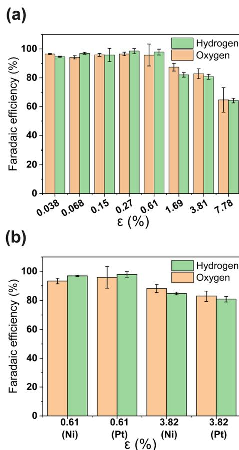
Fig. 3 (a) The faradaic efficiency for  $\text{H}_2$  and  $\text{O}_2$  of PSI-ZGEs with a pore diameter of  $4.1 \mu\text{m}$  at a constant current density of  $10 \text{ mA cm}^{-2}$  is shown for separators of different porosities. (b) The faradaic efficiency for  $\text{H}_2$  and  $\text{O}_2$  with Pt, and Ni electrocatalysts are compared at  $\epsilon = 0.61\%$  and  $\epsilon = 3.82\%$  porosity. All error bars indicate one standard deviation about the sample mean.
