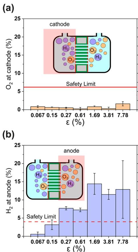
Fig. 4 (a) and (b) Show the relative concentrations of  $O_2$  in the cathodic gas outlet and  $H_2$  in the anodic gas outlet streams. In (a) and (b) outlet pressure was  $1.3\text{ bar}$ . The flammability limits of  $H_2$  and  $O_2$  mixtures are indicated as horizontal lines.<sup>38</sup> In panels (a) and (b) gas concentrations are expressed as volume percentages. All error bars indicate one standard deviation about the sample mean.
