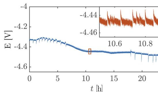
Fig. 5 Variation of cell voltage with time recorded during a chronopotentiometry experiment performed with a platinum-coated PSi-ZGE with a pore size of  $4.1\text{ }\mu\text{m}$  and porosity of  $0.61\%$  at a constant current of  $100\text{ mA cm}^{-2}$  shows that PSi-ZGE does not materially degrade over the  $24\text{ h}$ . The fluctuations in potential due to bubble evolution are made clearer in the inset.
