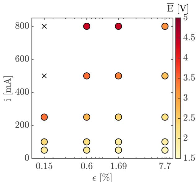
Fig. 7 The average cell potential is shown for different currents and PSi-ZGE porosities at an electrolyte flow rate of  $100 \text{ mL min}^{-1}$ . The color of the points indicates the magnitude of the average potential (see colorbar). The black crosses indicate combinations of current and porosity that were not possible to achieve because the cell potential exceeded the 5 V limit imposed on the potentiostat.
