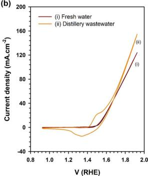
Fig. 3 (a) Linear sweep voltammogram results of stainless steel and  $\rm Ni_2Se_3$  nanoparticles coated stainless steel substates in freshwater and distillery wastewater electrolyte. (b) CV of  $\rm Ni_2Se_3/SS$  anode in freshwater and distillery wastewater-based electrolyte. Note that the concentration of the electrolyte was 1 M NaOH.
