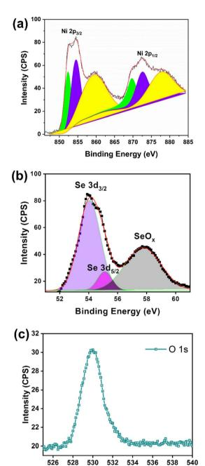
Fig. 2 (a) High resolution of Ni 2p, (b) Se 3d, and (c) O 1s spectra of XPS using the as-synthesized Ni<sub>2</sub>Se<sub>3</sub> powder sample.
