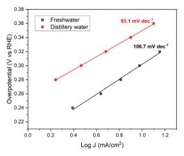
Fig. 4 Tafel plots of Ni<sub>2</sub>Se<sub>3</sub> in freshwater and distillery wastewater electrolytes.
