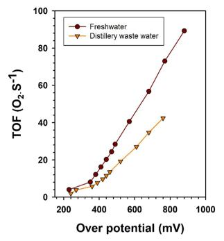
Fig. 7 TOF of Ni<sub>2</sub>Se<sub>3</sub>/SS anode in electrolytic oxygen generation performance in fresh water and distillery wastewater.
