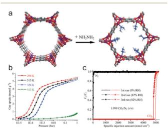
Fig. 40 (a) Introducing  $N_2H_4$  into pores of  $Mg_2(dobdc)$ . (b) The  $CO_2$  sorption isotherms of  $(Mg_2(dobdc)(N_2H_4)_{1.8})$  at different temperatures. (c) The breakthrough curves of  $(Mg_2(dobdc)(N_2H_4)_{1.8})$  for  $CO_2/N_2$  (1: 999) under different humid conditions. Reproduced from ref. 223 with permission from the Royal Society of Chemistry, Copyright 2016.
