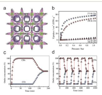
Fig. 42 (a) The structure of UTSA-280. (b) The CO<sub>2</sub>/CH<sub>4</sub> sorption isotherms of UTSA-280 at 273 and 298 K. (c) and (d) The breakthrough curves and cycles of UTSA-280 for  $CO_2/CH_4$  (1:1). Reproduced from ref. 245 with permission from Wiley, Copyright 2020.
