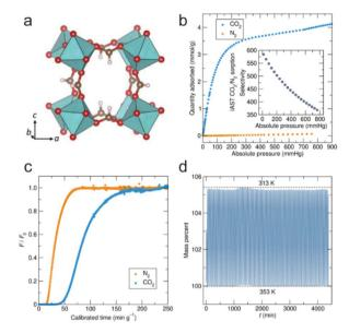
Fig. 31 The structure and  $CO_2$  adsorption performance of ALF. Reproduced from ref. 210 with permission from the Advancement of Science, Copyright 2022. (a) The structure of ALF. (b) The  $CO_2/N_2$  sorption isotherms of ALF at 298 K. (c) The breakthrough curves of ALF at 323 K. (d) 130 cycles of adsorption and desorption.
