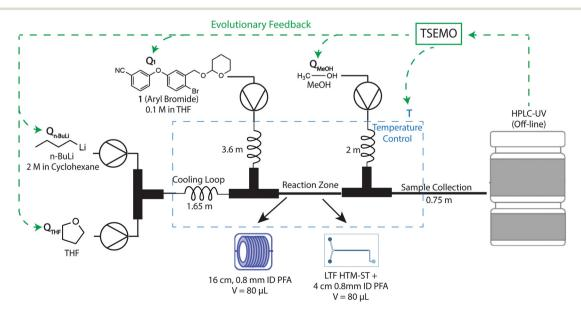
Fig. 1 A schematic representation of rector setup to perform machine learning-driven optimization of the lithium-halogen exchange of reaction given in Scheme 1b
