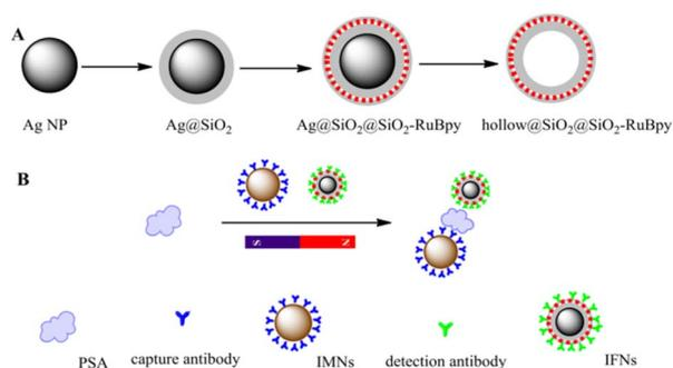
Fig. 9 (A) Schematic illustration for synthesis of Ag@SiO<sub>2</sub>@SiO<sub>2</sub>-RuBpy and hollow@SiO<sub>2</sub>@SiO<sub>2</sub>-RuBpy. (B) Schematic illustration for the construction of the detection of PSA with the immunomagnetic nanospheres and immunofluorescent NPs. Reprinted with permission from ref. 111 Copyright (2017) Elsevier.
