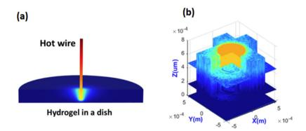
Fig. 8 Ultrabright fluorescent nanothermometers- nanoparticles allow measuring 3D mapping of temperature distribution. (a) 3D temperature distribution of a heated wire in hydrogel simulated with a stationary numerical model solution. (b) 3D temperature measurements using nano-UMSP. [Reproduced from ref. 30 with permission from RCS, copyright 2021.].
