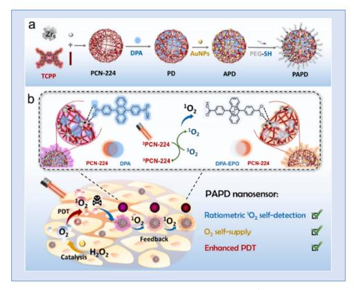
Fig. 25 Representation of (a) PAPD preparation and (b) multifunctional integration of ratiometric  ${}^{1}O_{2}$  self-detection,  $O_{2}$  self-supply and enhanced PDT. Reproduced with permission. Elsevier.
