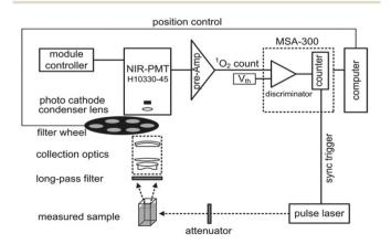
Fig. 5 Schematic diagram of the time- and wavelength-resolved  $^1{\rm O}_2$  luminescence detection system. $^{20}$
