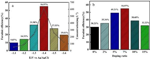
Fig. 35 The FE of CO<sub>2</sub> reduction to formate was investigated using a carbon paper electrode loaded with 7%-(Cu, N)-SnO<sub>2</sub> at various potentials (a). The faradaic efficiency of  $CO_2R$  to formate was studied using different electrodes with varying amounts of (Cu, N) doping at a potential of -1.4 V, with an electrolysis time of 1 hour (b). Reproduced with permission from ref. 375. Copyright 2020, Elsevier.
