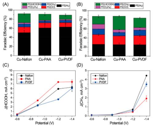
Fig. 31 The  $CO_2RR$  performance of various Cu/C catalysts with different binders was evaluated. The FE of HCOOH, CO, CH<sub>4</sub>,  $C_2H_4$ , and H<sub>2</sub> was evaluated at two different potentials: -0.6 V and -1.4 V (A and B). The partial current density profiles of HCOOH and CH<sub>4</sub> are presented (C and D). Reproduced from ref. 339. Open access article, American Chemical Society.
