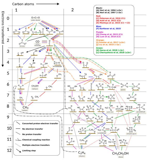
Fig. 3 Possible different routes for the production of C<sub>1</sub> and C<sub>2</sub> products over the surface of polycrystalline copper upon e-CO<sub>2</sub>R. Reproduced with permission from ref. 11. Copyright 2023, American Chemical Society.
