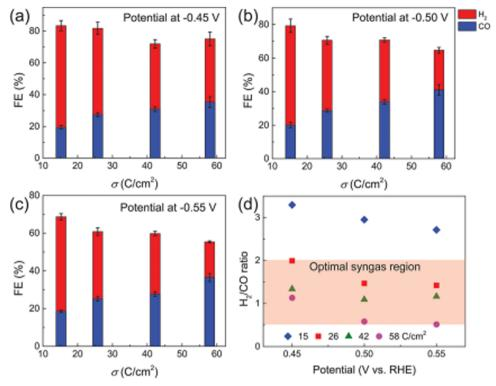
Fig. 30 The FEs of H<sub>2</sub> and CO production on OD-Cu NPs were measured at different applied potentials: (a) -0.45 V, (b) -0.50 V, and (c) -0.55 V. The controllable composition of syngas varies depending on the applied potentials (d). Reproduced with permission from ref. 331. Copyright 2020, American Chemical Society
