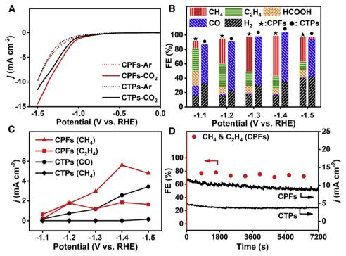
Fig. 26 e- $CO_2R$  performance of carbon-based transition metal catalysts (CTPs) and carbon-based precious metal-free catalysts (CPFs) was evaluated by LSV curves at a scan rate of 10 mV s<sup>-1</sup> in both Ar- and  $CO_2$ -saturated solution (A). The FEs of various products (B). The partial current densities of various products (C). The FE and current density of CPFs and CTPs were measured at a potential of 1.4 V *versus* RHE (D). Reproduced from ref. 261. Open access article, Elsevier.
