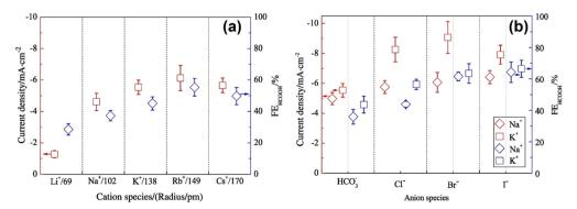
Fig. 37 Current density and  $FE_{HCOOH}$  as functions of electrolyte type and the cation size, measured using an  $SnO_2/C$  electrode at -1.4 V in 0.1 mol  $L^{-1}$  MHCO<sub>3</sub> (M =  $Li^+$ ,  $Na^+$ ,  $K^+$ ,  $Rb^+$ ,  $Cs^+$ ) and NaX and KX (X =  $HCO_3^-$ ,  $Cl^-$ ,  $Br^-$  and  $I^-$ ), respectively (a and b). Reproduced with permission from ref. 413. Copyright 2020, Elsevier.
