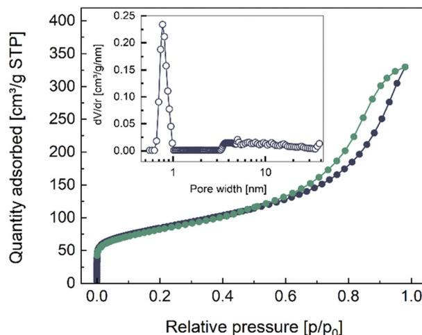
**Fig. 2**  $\text{N}_2$  adsorption (black) and desorption (green) isotherms of the  $\text{Ti}_9\text{O}_{17}$  nanowires synthesized in saturated KOH *via* electrochemical erosion. The inset shows the pore size distribution with a strong peak around  $\sim 0.8$  nm.
