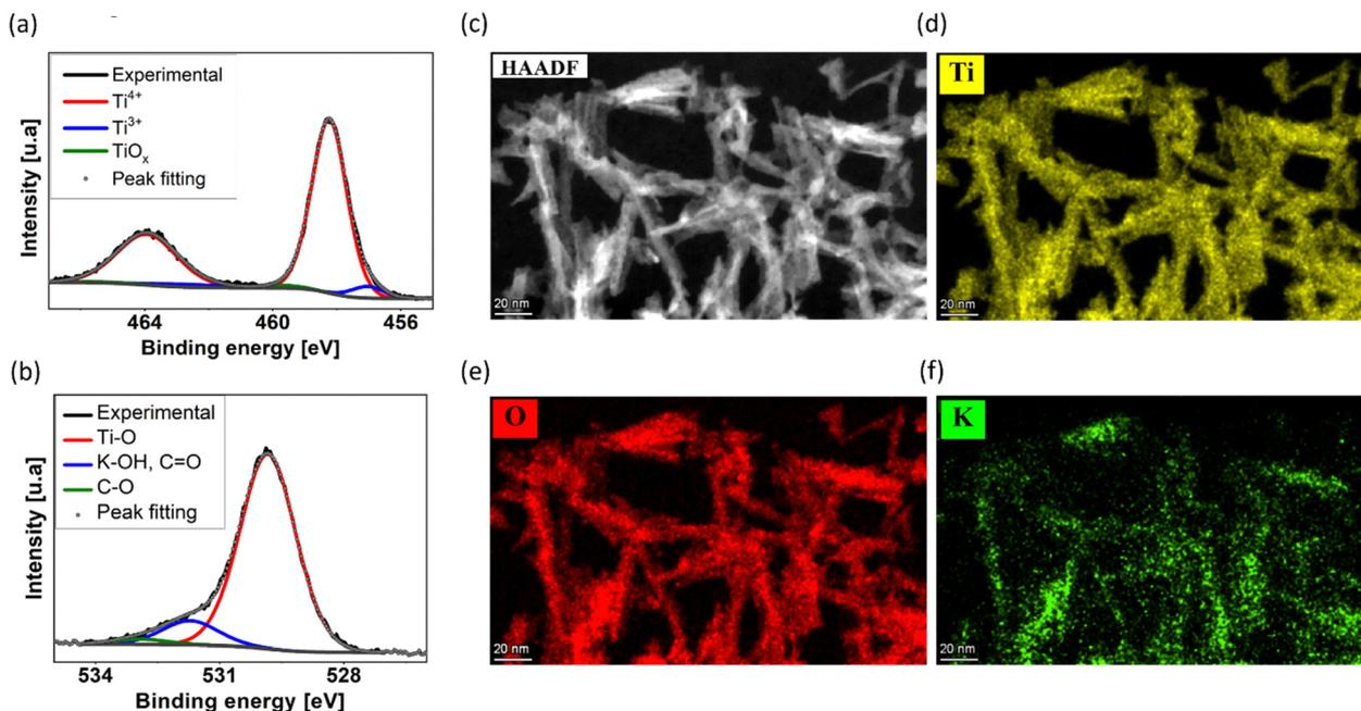
Fig. 3 (a) and (b) XPS spectra of the synthesized nanowires with the  $2p_{1/2}$  and  $2p_{3/2}$  doublet peaks for Ti 2p and O 1s, respectively. The peaks indicate the presence of Ti with different oxidation states. (c) STEM-HAADF image of a nanowire network. (d), (e) and (f) corresponding STEM-EDX elemental maps of nanowires for Ti–K, O–K, and K–K, respectively.
