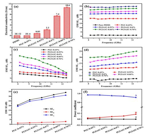
Fig. 10 (a) Electrical conductivity and (b) SE<sub>T</sub> of PDMS, PGC-0.43% and PGACs in the X-band, (c) SE<sub>R</sub>, (d) SE<sub>A</sub>, (e) the average SE<sub>T</sub>, SE<sub>R</sub>, SE<sub>A</sub>, and (f) the average power coefficients (A, R, T) of PGC-0.43% and PGACs in the X-band; reproduced with permission from ref. 94, copyright reserved Elsevier 2019.
