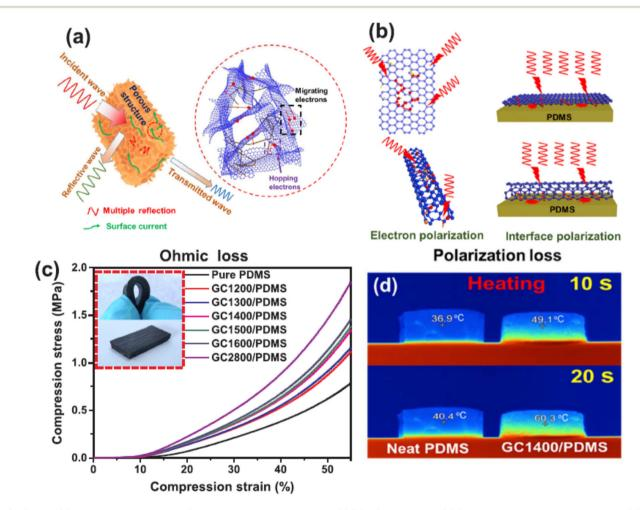
Fig. 8 (a and b) Schematic diagram of the EM shielding mechanism of the GC/PDMS composites. (c) Compression stress-strain curves of GC1400/ PDMS and neat PDMS. The inset shows the optical images of GC1400/PDMS and the bent GC1400/PDMS. (d) Infrared thermography images of GC1400/PDMS and neat PDMS in heating for 10 s and 20 s (the hot stage with a temperature of 150 °C); reproduced with permission from ref. 90, copyright reserved Elsevier 2020.
