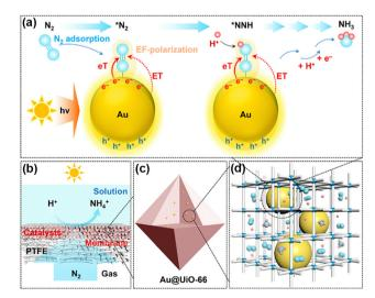
Fig. 10 Schematic illustration for direct PNRR on Au@UiO-66. (a) Illustration of the direct PNRR on AuNPs. (b) Schematic of the GMS reaction interface design. (c) and (d) Schematic diagram showing the dispersion of plasmonic AuNPs within the cavities of the MOF matrix. Reprinted with permission from ref. 127. Copyright 2021 American Chemical Society.
