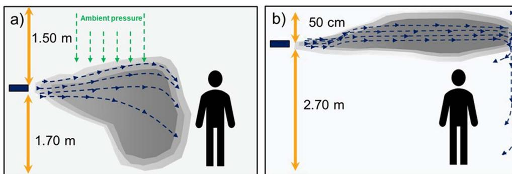
Fig. 1 Comparison of dosing  $O_3$  gas,  $H_2O_2$ , or TEG aerosols into the office room at (a) a medium height of about 1.5 m (without the Coandă effect), and (b) at 50 cm from the ceiling (at a height of 2.5 meters) with the Coandă effect.
