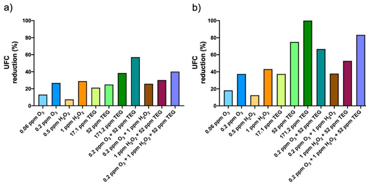
Fig. 3 Percentage of UFC reduction of (a) bacteria and (b) fungi over surfaces with triethylene glycol (TEG), ozone (O<sub>3</sub>) and hydrogen peroxide (H<sub>2</sub>O<sub>2</sub>) nebulized individually and combined. Plots represent percentage of reduction relative to the bacteria and fungi present before the nebulization of the compounds.
