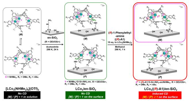
Scheme 1 Preparation of a supported helical LCo<sub>3</sub> complex, LCo<sub>3</sub>((R)-A1)/en-SiO<sub>2</sub>, by grafting of [LCo<sub>3</sub>(NHMe<sub>2</sub>)<sub>6</sub>](OTf)<sub>3</sub> on an ethylenediaminefunctionalized SiO<sub>2</sub> surface (en-SiO<sub>2</sub>), followed by the addition of chiral (R)-1-phenylethylamine. Possible paired surface structures are presented. The whole scheme for LCo<sub>3</sub>((R) or (S)-A1)/en-SiO<sub>2</sub> is presented in the ESI† (Scheme S1).
