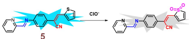
Fig. 8 Proposed sensing mechanism of 5 with \text{ClO}^- ions.
