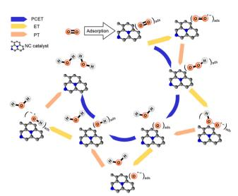
Fig. 7 Representative possible elementary steps during four-electron ORR ( $O_2 + 4H^+ + 4e^- \rightarrow 2H_2O$ ) on carbon-based electrocatalysts. Black and blue balls represent carbon and nitrogen atoms, respectively. Reprinted with permission from ref. 210. Copyright 2018 American Chemical Society.
