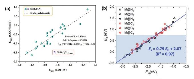
Fig. 2 (a) Scaling relationship between the adsorption energy of \*CO and \*COOH. Reprinted with permission from ref. 129. Copyright 2021 Royal Society of Chemistry. (b) The scaled relationship between the activation energy and adsorption energy of H atom (BEP relationship) was examined on single-atom catalysts. Reprinted with permission from ref. 130. Copyright 2021 Royal Society of Chemistry.
