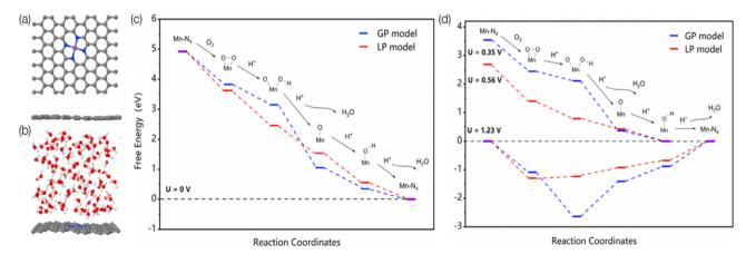
Fig. 5 The surface models of  $MnN_4$ -graphene in the (a) gas-phase (GP) and (b) liquid-phase (LP) model. The Mn, C, N, O, and H atoms are represented in purple, gray, blue, red, and white, respectively. Predicted free-energy pathways for ORR under different electrode potentials at pH = 0. (c) U = 0 V. (d) U = 1.23 V for both GP and LP models, U = 0.35 V for the GP model, and U = 0.56 V for the LP model. Reprinted with permission from ref. 176. Copyright 2020 American Chemical Society
