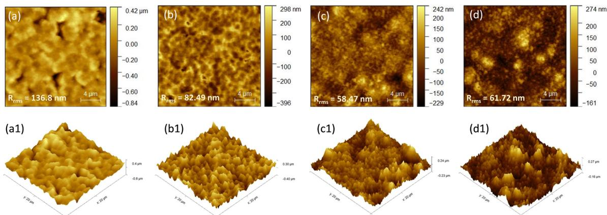
**Fig. 4** AFM images. (a) 2D and (a1) 3D AFM topography images of FACs film, (b) 2D and (b1) 3D AFM topography images of FACs film with TAEA with a volumetric concentration of 200 : 0.5, (c) 2D and (c1) 3D AFM topography images of FACs film with TAEA with a volumetric concentration of 200 : 1, and (d) 2D and (d1) 3D AFM topography images of FACs film with TAEA with a volumetric concentration of 200 : 1.5.
