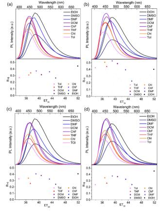
Fig. 2 Solvatochromic effects (top) and relative quantum yields (bottom) of NISCF-Xs in various solvents.
