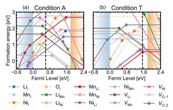
Fig. 5 Formation energies as a function of Fermi level for intrinsic defects in P4<sub>3</sub>32 LiMn<sub>1.5</sub>Ni<sub>0.5</sub>O<sub>4</sub> under (a) O-rich (the most intrinsically p-type) condition A and (b) O-poor (the most intrinsically n-type) condition T. The self-consistent Fermi levels are denoted by the black dashed lines. Interstitial defects (dotted lines) and antisite and vacancy defects (solid lines) with the lowest energy charge states are shown, for clarity,
