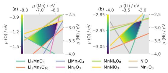
Fig. 3 The chemical potential space of  $P4_3$ 32 LiMn<sub>1.5</sub>Ni<sub>0.5</sub>O<sub>4</sub>, (a) where chemical potential of Li was set to an average value of -3.35 eV; (b) where chemical potential of Mn was set to an average value of -6.42 eV. Yellow/dark-blue colour shadings represent p/n-type conditions.
