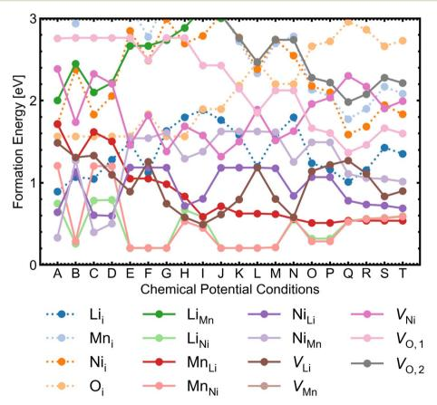
Fig. 4 Formation energies for each intrinsic point defect in the lowest energy charge state at the self-consistent Fermi levels over 20 chemical potential conditions for  $P4_332 \text{ LiMn}_{1.5}\text{Ni}_{0.5}\text{O}_4$ . The chemical potential conditions (A  $\rightarrow$  T) are arranged in order of increasing self-consistent Fermi level determined from all intrinsic point defects. Interstitial defects are represented by dotted lines; antisite and vacancy defects are shown by solid lines.
