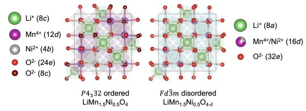
Fig. 1 Representative structures (with Wyckoff positions) of the  $P4_{\pi}32$  ordered and  $Fd\bar{3}m$  disordered LMNO
