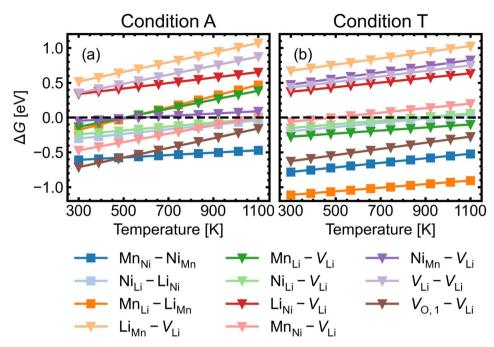
Fig. 7 Gibbs free energy change  $\Delta G$  for complex formation as a function of temperature under (a) the most intrinsically p-type O-rich condition A and (b) n-type O-poor condition T, using eqn (10). Stoichiometric complexes are denoted by squares and non-stoichiometric complexes are denoted by triangles. A negative  $\Delta G$  suggests complex association is likely, provided the constituent point defects are sufficiently mobile.
