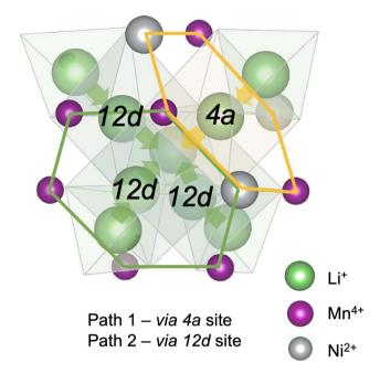
Fig. 10 A schematic showing 4a and 12d gate sites giving two distinct Li<sup>+</sup> migration paths in P4<sub>3</sub>32 LiMn<sub>1.5</sub>Ni<sub>0.5</sub>O<sub>4</sub>. The 4a site surrounded by 3Mn<sup>4+</sup> and 3Ni<sup>2+</sup>; the 12d sites surrounded by 5Mn<sup>4+</sup> and a Ni<sup>2+</sup>. Path 1 and path 2 are denoted by yellow and green arrows, respectively. Oxygen atoms which define the polyhedral vertices are not shown for
