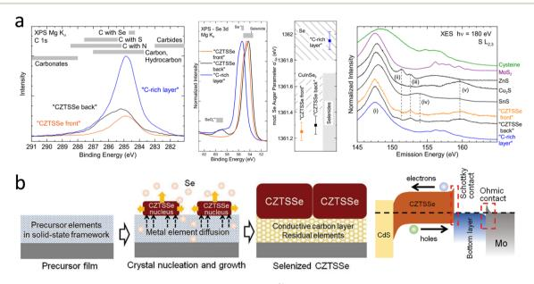
Fig. 3 (a) C 1s XPS, Se 3d XPS, and XES spectra of the investigated samples.<sup>64</sup> Reproduced with permission from ref. 64. (b) Schematic diagrams of the TGA-ammonia method and the energy-band structure of the cell.<sup>63</sup> Reproduced with permission from ref. 63.
