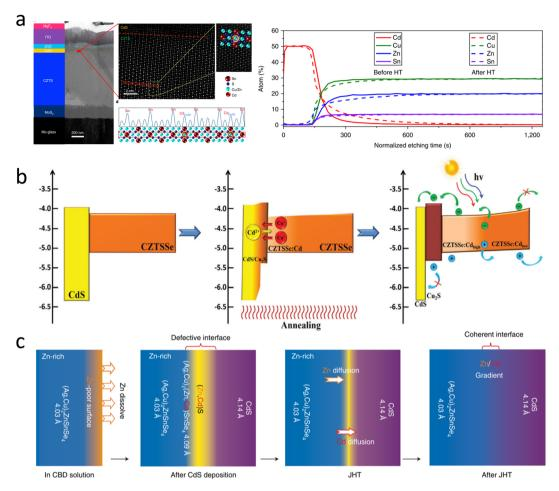
Fig. 9 (a) TEM cross-section of a CZTS device using the HT process, with the corresponding device structure shown on the left. 108 Reproduced with permission from ref. 108. (b) Schematic of the energy-band structure and the diffusion of Cu<sup>+</sup> and Cd<sup>2+</sup> ions during heterojunction annealing.<sup>40</sup> Reproduced with permission from ref. 40. (c) Schematic of the diffusion of the ions during heterojunction annealing.<sup>32</sup> Reproduced with permission from ref. 32
